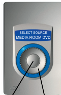
Press briefly to make source selection. Turn left or right to scroll through source list.
