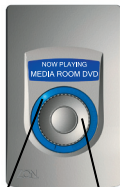
Virtual Pointer™ shows current volume level. Use jog wheel to adjust volume.
